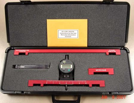
Profiles can be assessed quickly and accurately by sliding the digital gauge along the bridging bar. Notched feet and ceramic magnets prevent the bridge from rocking on the pipe. The magnets securely hold the bridge in place which makes it ideal when working upside down. Locking adjustment screws allows instant calibration to reference surface. Pointed and needle tips find the deepest section of pits with ease.
