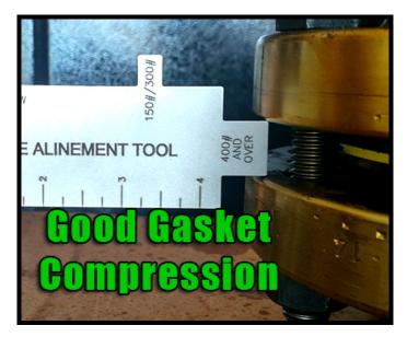
If the nib enters the space between the two flanges then it is considered to have Bad Gasket Compression and will need to be checked for additional bolt stress.
